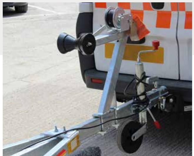
Fully welded and hot dip galvanised, SBS trailers are manufactured this way to ensure they're resistant to corrosion.
